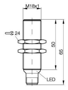
Inductive Sensors BES M18MI-PSC50B-S04K M18x1 x 65 normally-open Sn=5mm shielded
